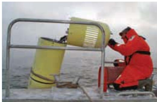
■ **Modern, plastic buoys have longer maintenance intervals and aren't 'ship wreckers' if there's contact**
